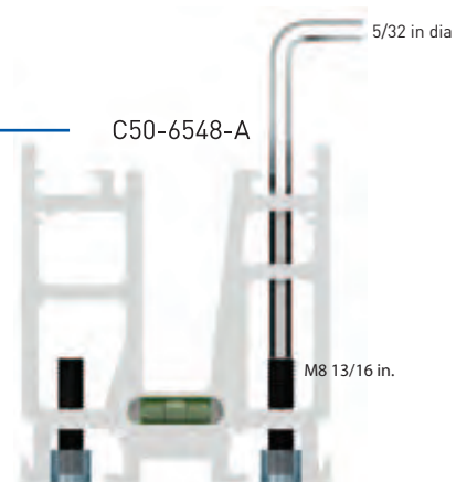
Adjustable block option for unlevel ground
